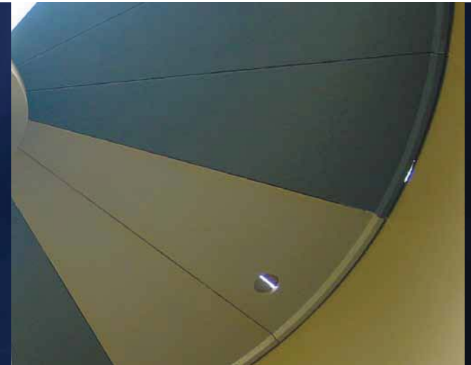
Right: Spray-on polyurethane coating in a processing tank
