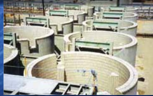
Above: Reactors lined with ceramic wear-and-tear protection
