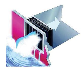
Munters Mist Eliminators allow inlet air to turn and pass between the profiles with minimum restriction. Drops impact the profile surface where they are collected and drained.
