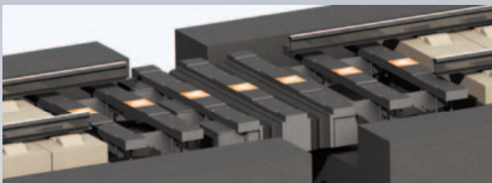
MAURER Guided Cross Tie System (400 mm longitudinal movement)
