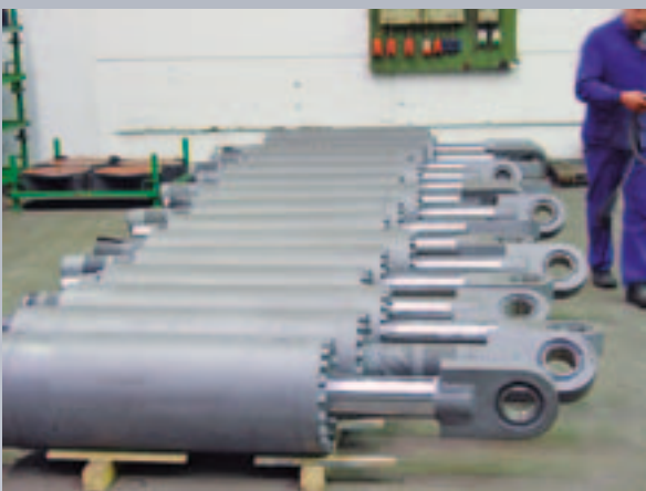
MAURER hydraulic dampers with 2,500 kN design force and 700 mm movement capacity for the Domovinski Bridge in Croatia
